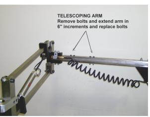
TELESCOPING 12 GA STEEL TUBING PERMITS EASY LENGTH ADJUSTMENT WHILE MAINTAINING STRENGTH INTEGRITY
